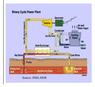
temperatures. In these locations *binary cycle* systems can be used. A binary cycle plant passes the geothermal water through a loop called a heat exchanger and the thermal energy is transferred to a working fluid (usually isobutane) that boils at a low temperature. The vapor from the working fluid is then used to drive turbine systems and generate electrical power.
